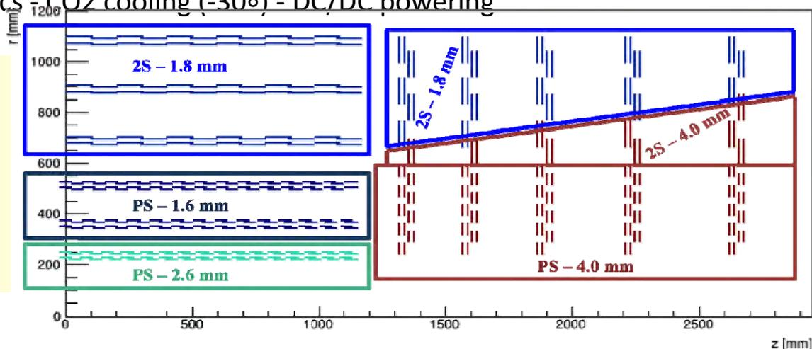
Ongoing study of alternative design with tilted modules in PS layers
