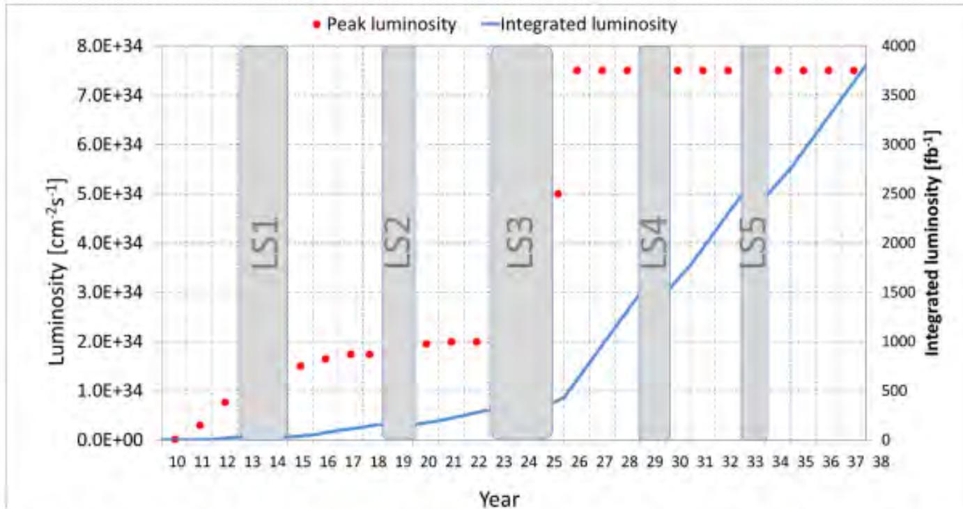
**Figure 8: Forecast for peak luminosity (red dots) and integrated one (blue line) in the HL-LHC era, for the case of ultimate HL-LHC parameters. Note that for sake of simplicity there is no learning curve for the luminosity after LS3.**
